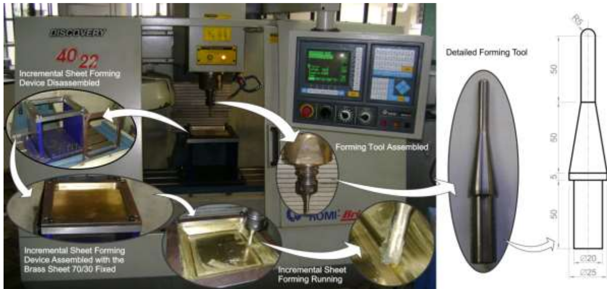
Fig. 5: Machining Center, device and tool for incremental forming used in the experiments.
