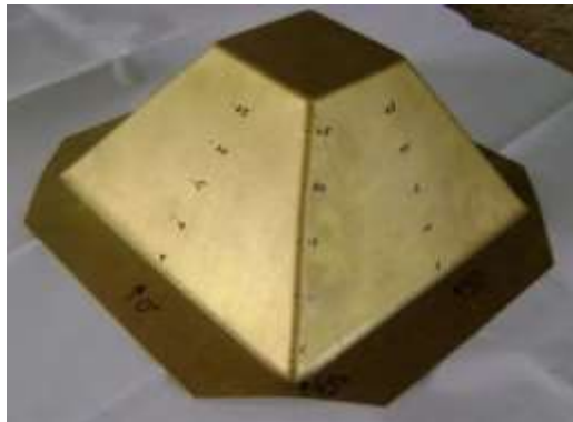
Fig. 10: Experiment 10 without fractures during ISF ( \Psi : 56^\circ | \Delta_z : 1,00 mm).
